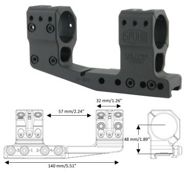
The mounts are machined from billet 7000-series aluminum and all aluminum parts are hardcoat anodized. The Torx 20 ring and clamping screws are zinc-nickel coated for corrosion resistance and come pre-waxed from the factory to ensure proper torque values.
