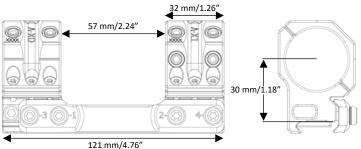
rings are diagonally cut for increased visibility of the elevation and windage turrets (US Patent 8,733,011).
