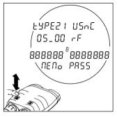
Use the azimuth key to scroll through the list.
