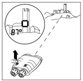
Sight the object with the pointing circle, then release the azimuth key while holding the VECTOR steady.
