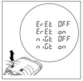
Click the azimuth key until the desired function status appears.
