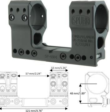
body to prevent canting of the rifle. The rings are diagonally cut for increased visibility of the elevation and windage turrets (US Patent 8,733,011).
