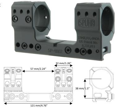
rings are diagonally cut for increased visibility of the elevation and windage turrets (US Patent 8,733,011).
